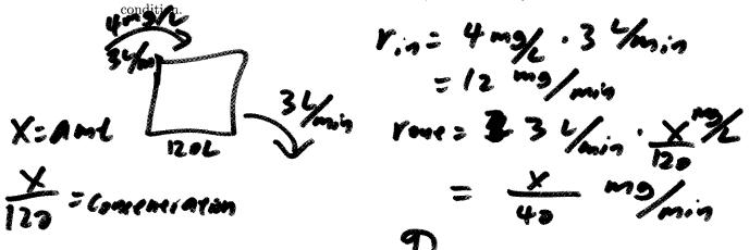
(b) (4 points) Use this system to find the concentration of ammonia in the tank as a function of time
