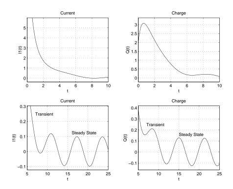
Note that the circuit's behavior, which appears to be exponential decay in the short term, turns out to be oscillatory in the long term. The apparent discrepancy arises because the circuit's behavior actually has two components: an exponential part that decays rapidly (the "transient" component) and an oscillatory part that persists (the "steady-state" component).
